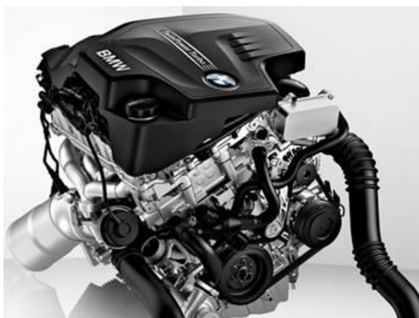
Fig 4 The award winning high efficiency 4-cylinder N20 engine
