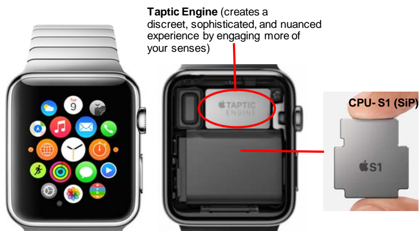
Fig. 3: Apple Watch has Force Touch function, and Taptic Engine is one of the key parts inside.
